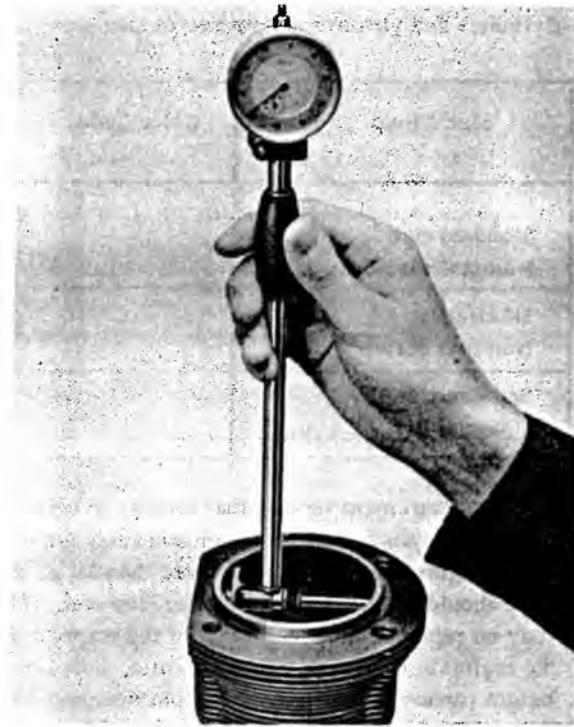
Checking cylinder bore.
