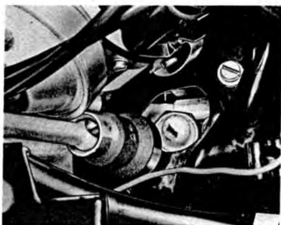
Oil cooler, checking for leaks
