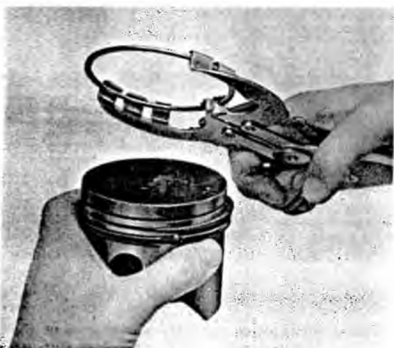
Piston rings, removing and installing
