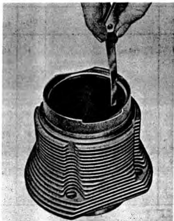
Checking piston ring end gap.
