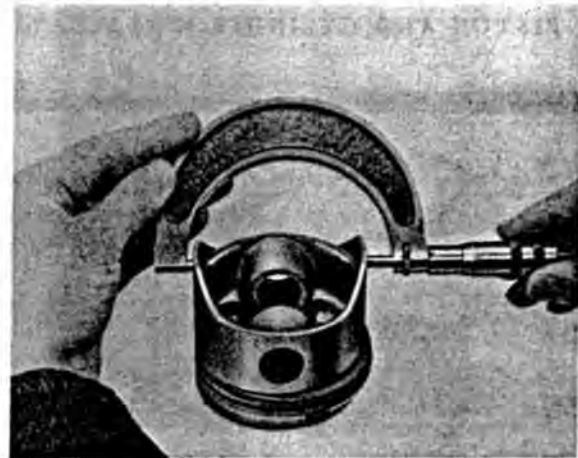
Checking piston diameter.
